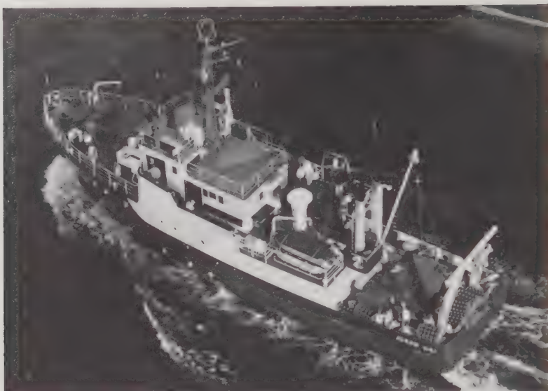
Fig. 3.01. Research cutter Alkor , a multipurpose vessel, 31 m in length, 236 gross tons, for research in the North Sea and the Baltic Sea (Photo: Institut für Meereskunde, Kiel).
