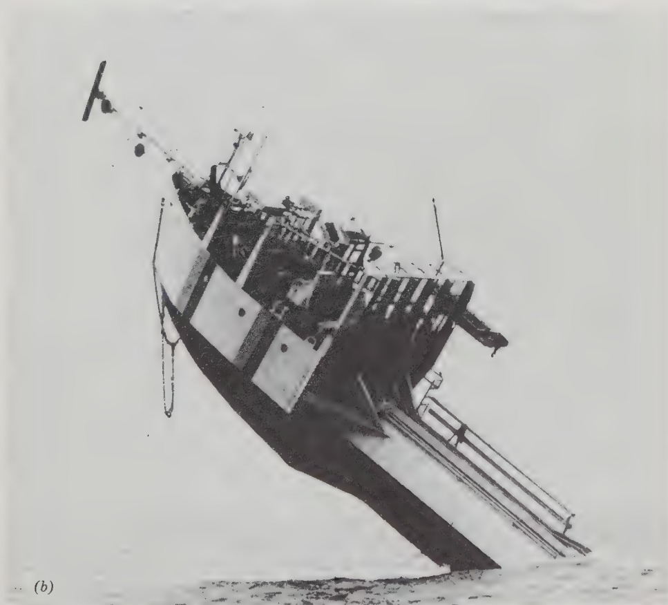
Fig. 3.12. The giant buoy Flip (Floating Instrument Platform) on her way to the operational area in horizontal position (a), while turning into the vertical position during the flooding of the ballast tanks (b), and in vertical position at the measuring site (c) (Photo: Scripps Institution of Oceanography, La Jolla).
