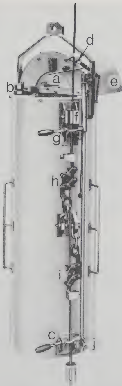
Fig. 3.17. 270-liter water bottle for sampling large amounts of water. During the lowering of the bottle, the water flows in through the cap, then along a separating wall to the bottom of the bottle from where it rises upwards and leaves the bottle through an opening which can be seen in front on top. When released by a messenger, the cover tips over and closes the bottle. In addition, the messenger is released to repeat the same process on the bottle following below. A high-pressure relief valve takes care of the pressure balance during the heaving of the instrument. Designations: (a) = cover, (b) = high-pressure relief valve, (c) = safety device for the wire, (d) = release lever, (e) = cap, (f) = clamping device for the wire, (g) = safety device for the wire, (h) = (i) = clamping device for the wire, (j) = release for series messenger (Studio photo: Hydro-Bios, Kiel).
