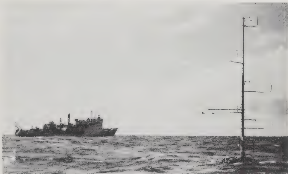
Fig. 4.02. Sensor-equipped buoy, stabilized by weight, for measurement of vertical profiles of wind, air temperature and humidity. Height of the mast 10 m, immersion depth of the buoy 4.5 m. In the background the research vessel Meteor in the tropical Atlantic during the Atlantic Trade Wind Experiment, 1969. (From Brocks, 1970.)
