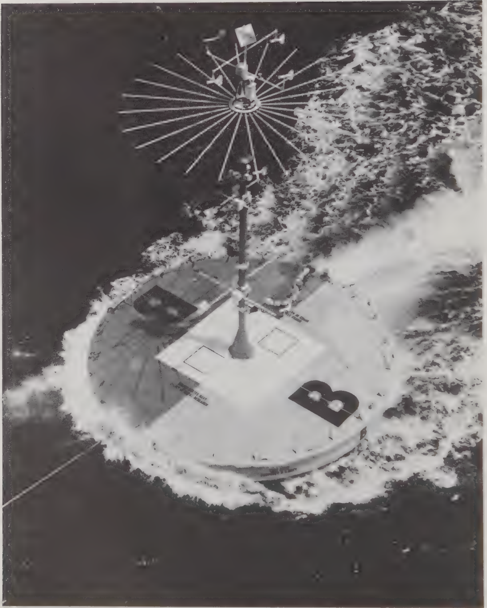
Fig. 3.14. Monster Buoy with measuring mast, arrays of sensors and antenna. Energy supply and electronic units are installed in the disk-shaped body of the buoy (Photo: General Dynamics, Convair Division).
